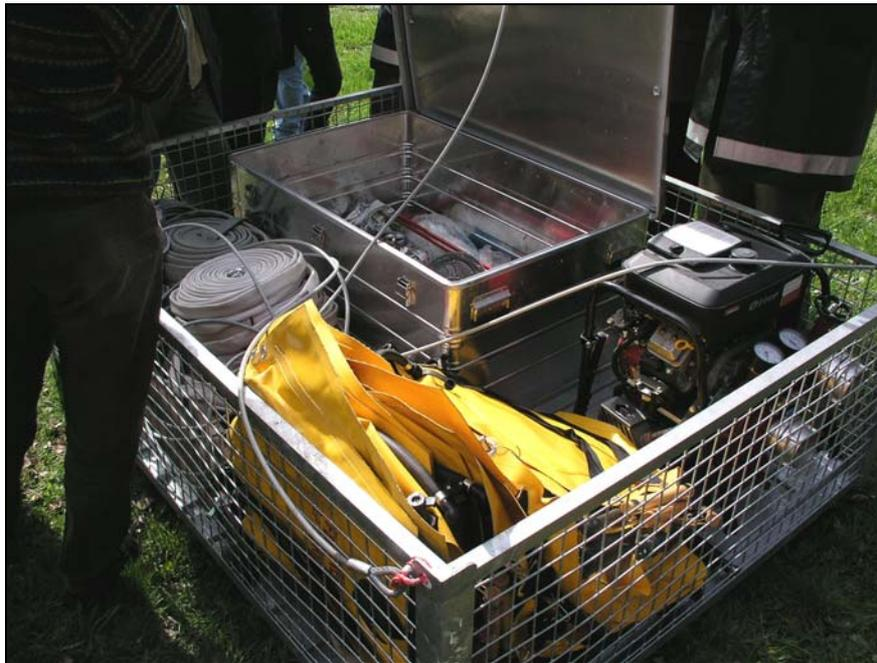
**Figure 5.** Forest fire box for the use at higher elevations with bad access or too long-lasting driving distances - to be transported with helicopter support.
