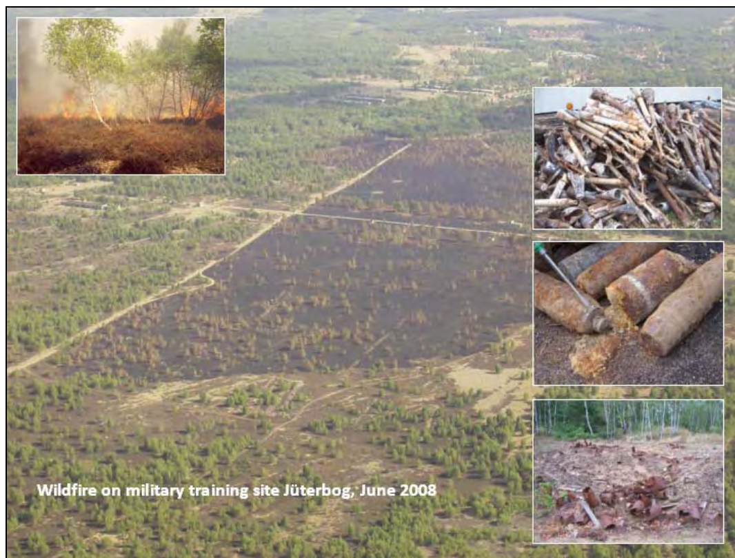
Figure 2. The „Heidehof-Golmberg“ conservation site requires the application of prescribed fire on ca. 1800 ha over the coming years. For the first time the project aims to use fire for halting succession and for regeneration of vegetation and at the same time facilitating UXO clearance. With the removal of dead and live vegetation layers the UXO becomes visible on the soil surface and can be cleared easier.
