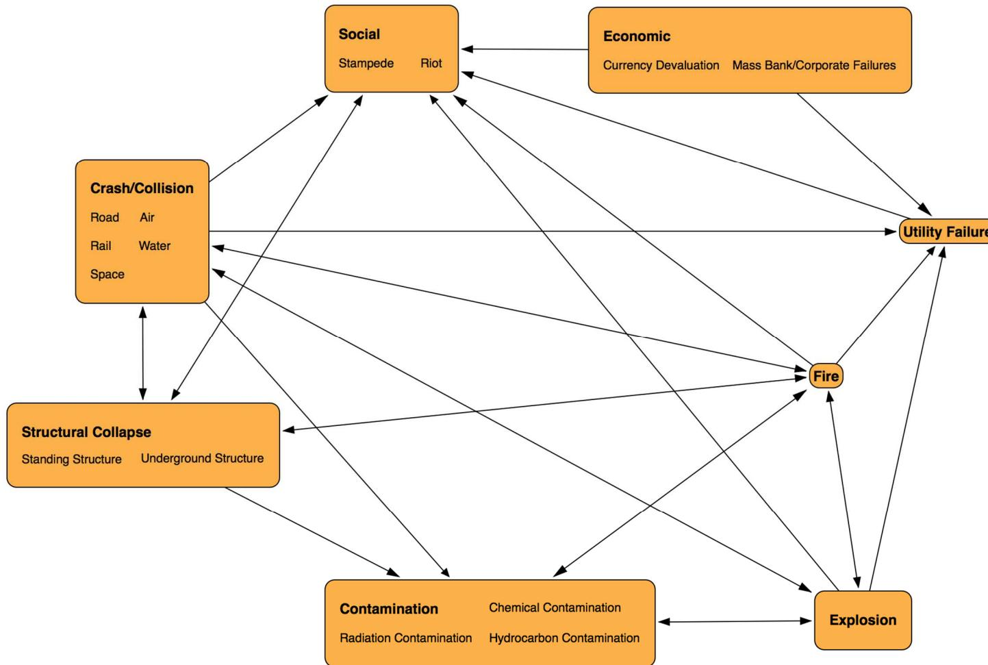
The causal loop diagram format makes it straightforward to draw connections between hazards. In this example, a crash/collision may cause contamination and so could an explosion, but contamination cannot cause a crash/collision, although it could cause an explosion. It would also be possible to integrate trigger events into the causal loop diagram format, but care must be exercised to ensure it does not become difficult to understand.
